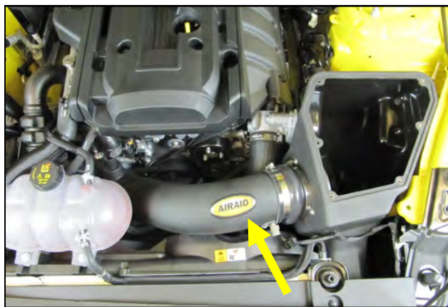
16. Insert the large end of the Intake Tube into the Hump Hose and tighten all 4 Intake Clamps at this time. Apply the Airaid Decal to the tube as shown.
