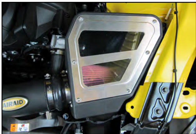
19. Remove the protective film from the Lid and Window before installation. Install the Airbox lid and Window onto the Airbox, with the Window on top, using 6 sets of 1/4" Button Heads and Washers.
